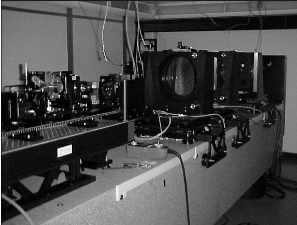
Figure 6 The NIST XCALIBIR interferometer is a state-of-the-art phase shifting interferometer capable of sub nanometer resolution.
