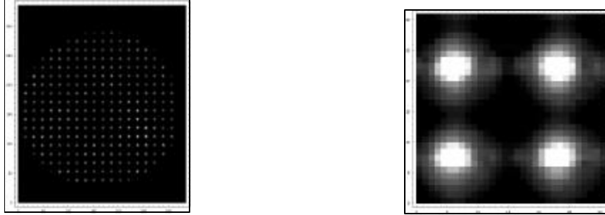
Figure 3.4: Normal eye, high resolution. The sample wavefront shown in the previous figure was used as an input function. The pupil in this case was 3.8 mm, with effective 210 \mu\text{m} resolution lenslets. The eye had a prescription of -3.75 -1.00 \times 16 . The first figure shows the image of the full eye, the second figure zooms in on four focal spots.
